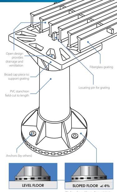
Wedge-shaped base discs rotate to accommodate floor slope.
